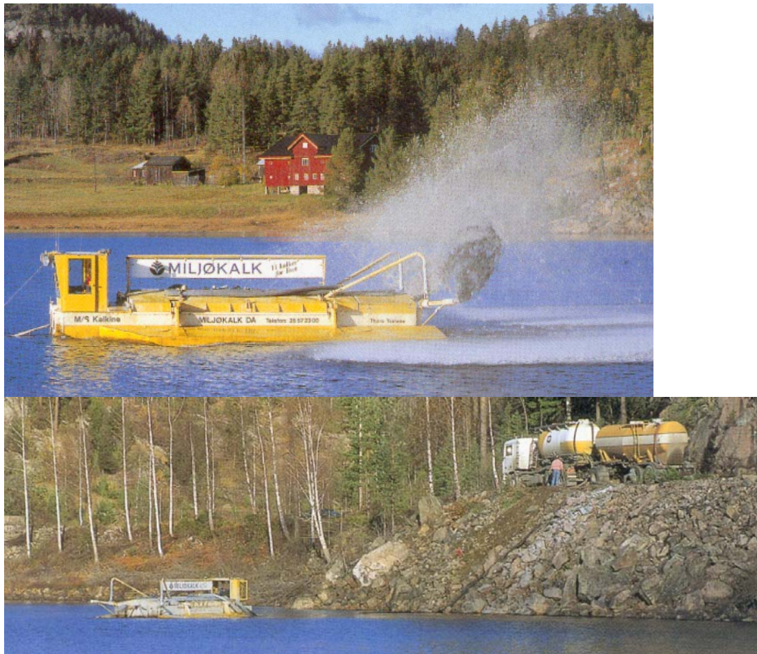
Figure 1. Lake liming. Limestone powder is transported by trucks to the lake, pumped to the spreading boat by air pressure, and then to the lake mixed with lake water to a slurry. (scanned with permission from http://www.norcem.no/kalk/ ).
