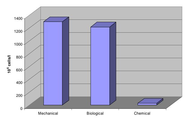
**Figure 17.** Algal growth potential expressed as cell yield of the green alga *Selenastrum capricornutum* in municipal wastewater after mechanical (primary), biological (secondary, activated sludge) and chemical treatment (precipitation with aluminium sulphate after primary treatment). The wastewater samples were diluted to 5% concentration in natural, oligotrophic lake water (data from Norwegian Institute for Water Research).
