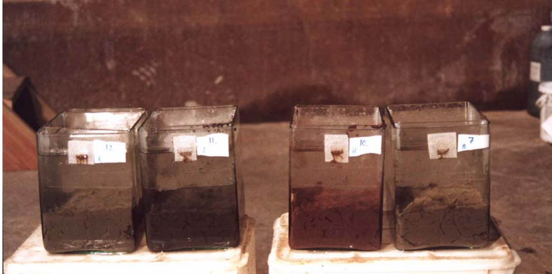
Figure 1. From left: Control (unspiked) sediment and sediment spiked with ilmenite, hematite and barite.
