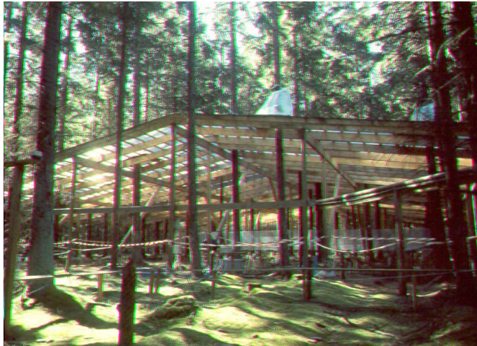
Klosterhede in Denmark – a 1200-m 2 roof built underneath the forest canopy to remove the acidic input to the soil and replace it with different combinations of clean rain and base cations (Beier et al. 1998).
