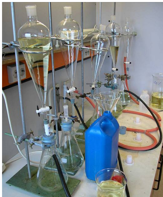
Figure 2. Apparatus used (five parallels) to retain \text{NO}_3^- from water samples on anion exchange resins. Photo: J.R.Selvik, NIVA.
