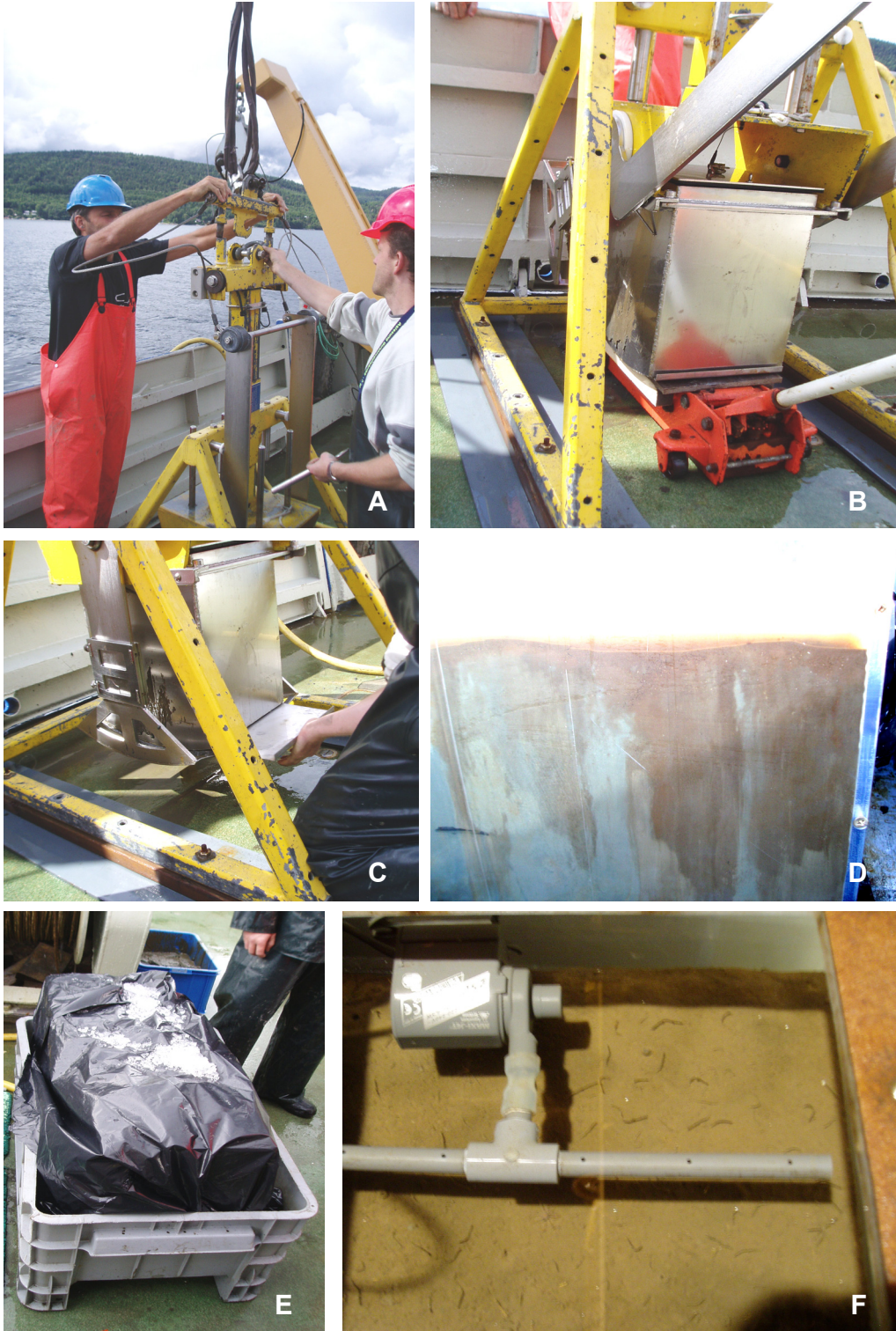
Figure 1. Box core sampling. A) Corer on deck with fresh sample. C) Insertion of bottom steel sheet. B) Spade opened and disconnection of steel box with internal liner. D) Internal liner with sediment sample removed from steel box. E) Storage on deck. F) Installed in mesocosm with pump for internal stirring (during operation the perforated pipe is bent down to discharge water jets parallel with sediment surface).
