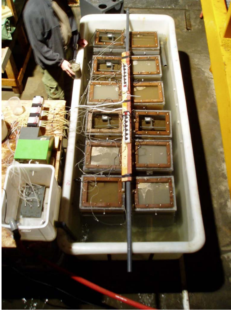
Figure 2. Test set-up showing header tank (down left), 15 channel peristaltic pump, and experimental boxes during addition of slurried particles.
