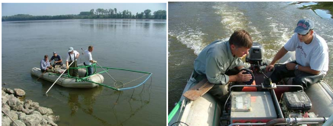
Figure 32. Electro-fishing (11 kW, 4 anodes, 30 Hp gasoline el-generator) device for test-fishing in large rivers. Likely to become EU-standard, and subsequent International-standard.
