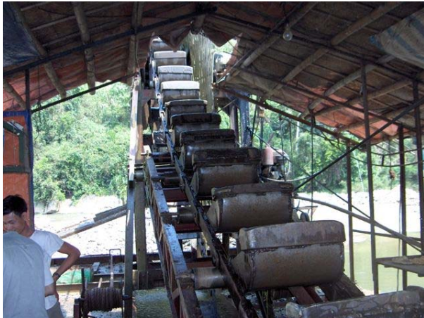
5. The material is transported up to a washing tower at the rear end of the barge
