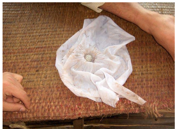
10. The result of four days and nights of gold washing. A lump of amalgam of the size of a ping pong ball. This is heated and the mercury vaporizes off, and the pure gold and some silver are left back. This last extraction is not performed on board the barge, but in town, we were told.
