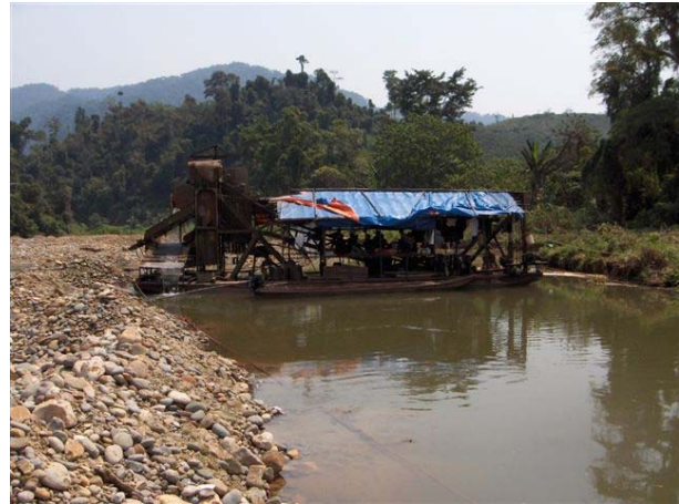
2. Eating old grass-covered banks in the front end, washing the material and spitting it out in the rear end
