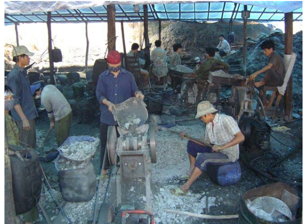
2. The ore is crushed to a particle size of fine sand and finer
