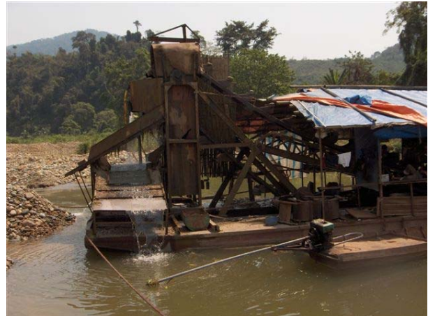
6. Here the material is separated, the stones and gravels are dumped backwards, while the sand and fine material go to both sides.
