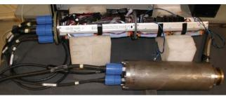
Figure 5: Electronic pressure case and its protection
