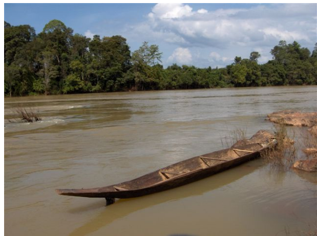
In Pum Phi at the border to Vietnam most boats were carved out of one single tree trunk and operated by paddles.
