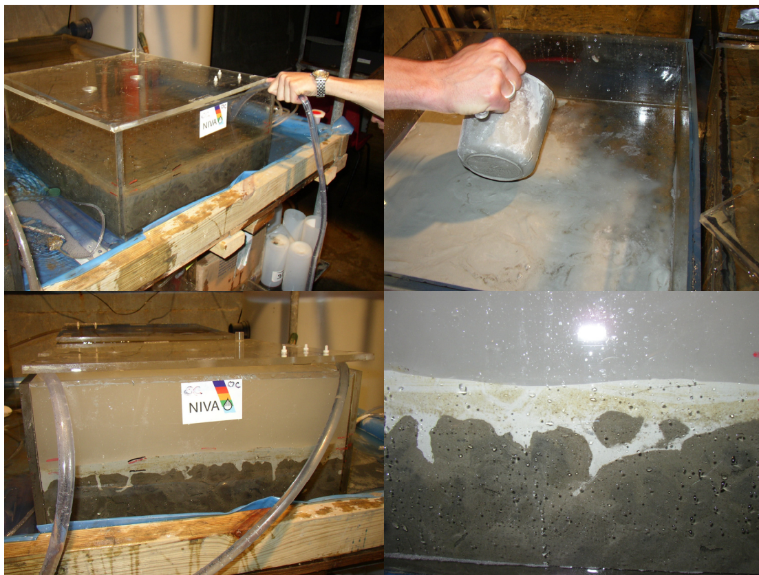
Figure 3. Removal of overlying water (top left), addition of olivine material (top right), addition of water to boxes (bottom left) and example of deposited olivine cap (bottom right)
