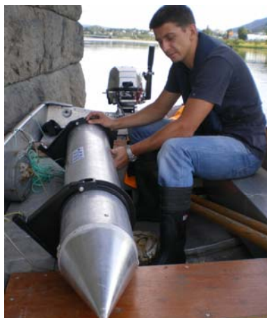
Figure 2-3. Deployment of the suspended sediment sampler in the Drammenselva River. The sampler was attached to a bridge pillar.
