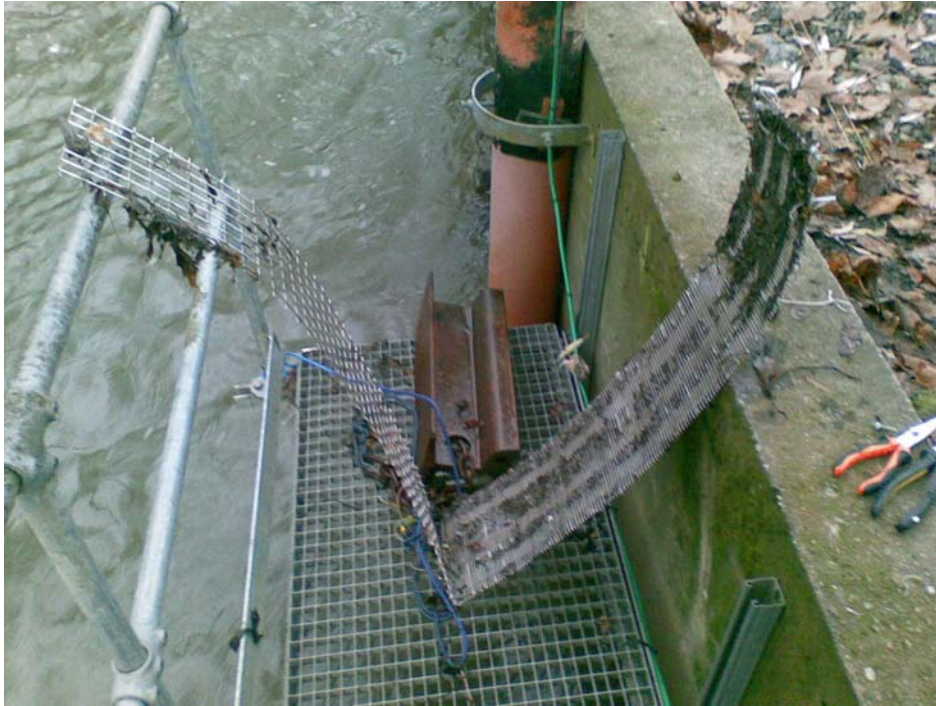
Figure 2-10. Deployment cage for the LDPE membrane and silicone samplers exposed in the Alna River. Note the wide stainless steel mesh allowing increased water turbulences around the samplers. This is likely to contribute to increasing uptake rates and lowering LODs.
