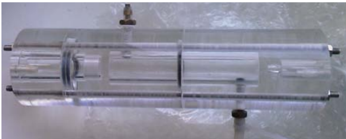
Figure 4.2.3 Flow cell for in situ pH measurements using at the Bjerknes Centre for Climate Research.
