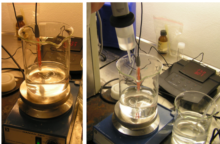
Figure 8. 1000 ml beaker on the magnetic stirrer with pH probe and 300 ml of Sol-0 ready for non purged titration. Right: showing addition of NaOH.
