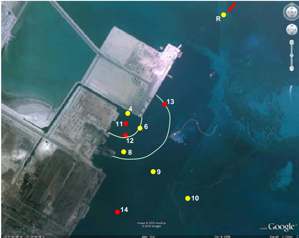
Figure 1. Suggested station positions for the 3 months survey. The URS stations included are shown in yellow with original station id-number, including the reference station (R). New stations are numbered from 11 and upward to avoid confusion with the other URS stations. Isolines describe the 250 m and 500 m distance from the discharge point.
