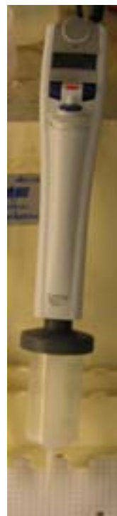
Figure 4. Eppendorf Multipette Xstream manual dispenser with a 50 ml syringe
