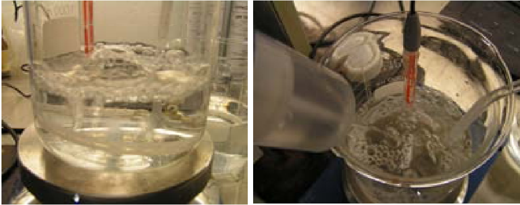
Figure 9. A 1000 ml beaker with magnetic stirrer, air purging running, pH probe and 300 ml of Sol-0 ready for titration with purging.
