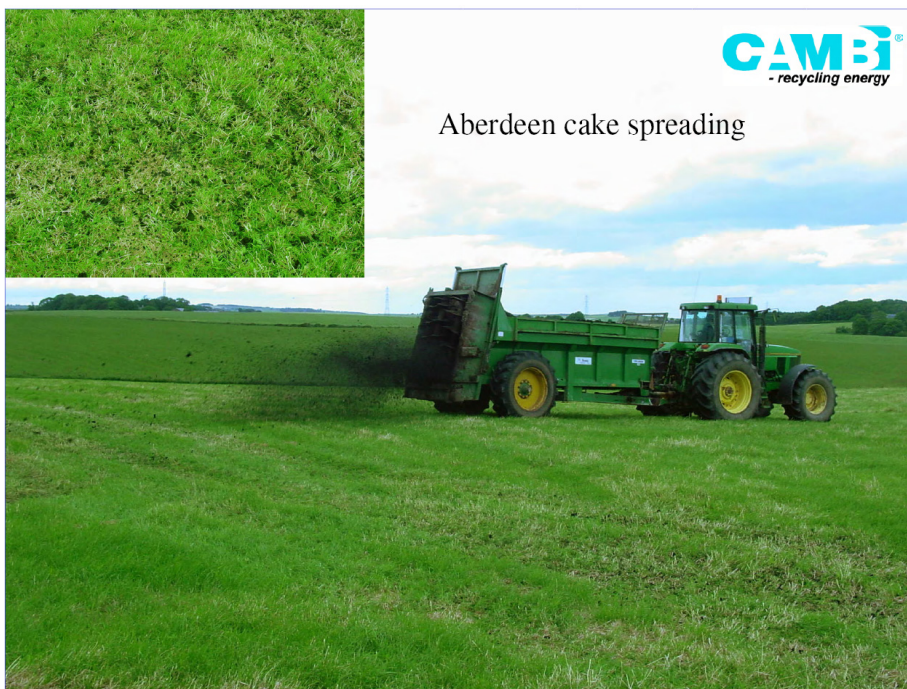
Figure 35. Dewatered digested biosolids from Aberdeen sludge treatment plant are spreading over the grassland in UK (Panter 2009)
