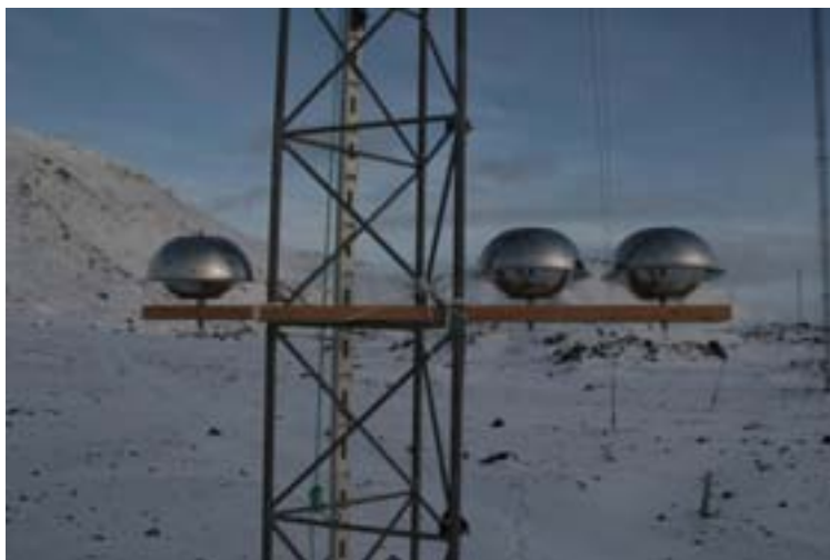
Figure 4. Passive PUF air samples at Bjørnøya
