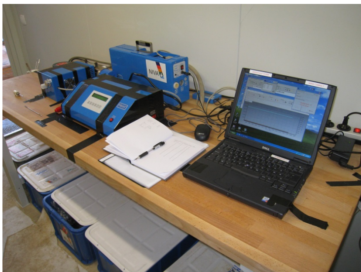
Picture C. The Lumex Mercury Analyzer with pyrolyzer unit (Photo: Sigurd Øxnevad).
