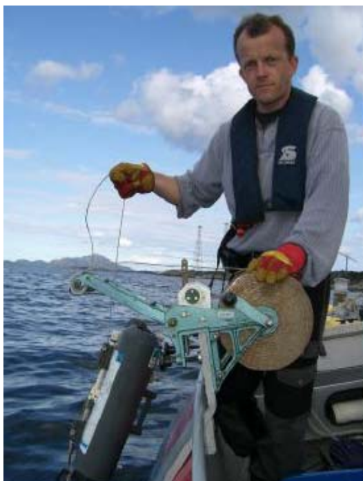
Figure 2. A Niskin water sampler was used to collect the water samples for particulate analysis (photo: Merete Schøyen).
