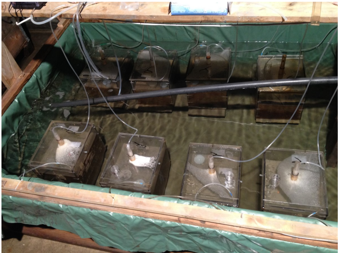
Figure S3. Photo of the boxcosm experimental setup depicted in the schematic in Figure S1 showing the four uncapped (front row) and capped (back row) sediment boxcosms
