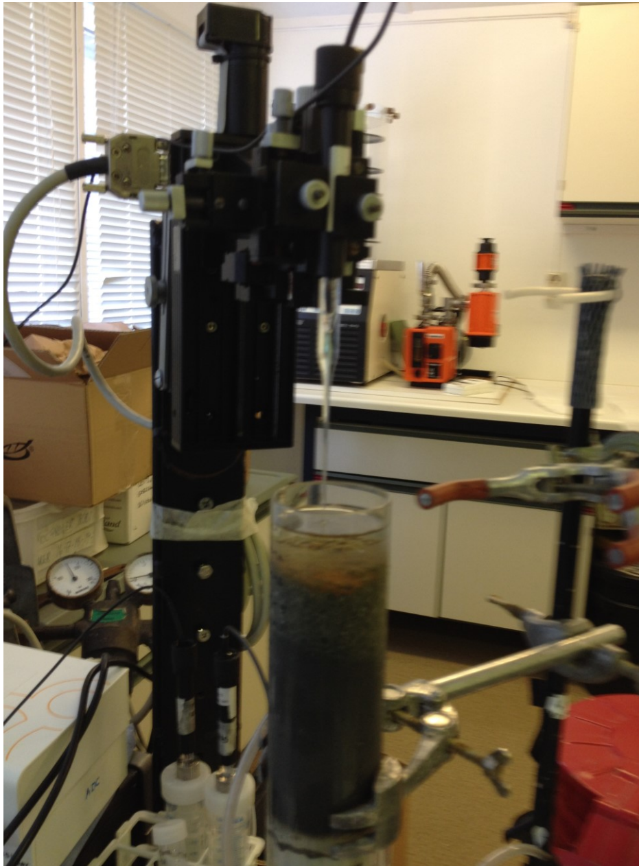
Figure S4. Set up for microsensor depth profile measurements of O_2 , H_2S and pH, showing O_2 concentration measurement on a core extracted from one of the boxcosms.
