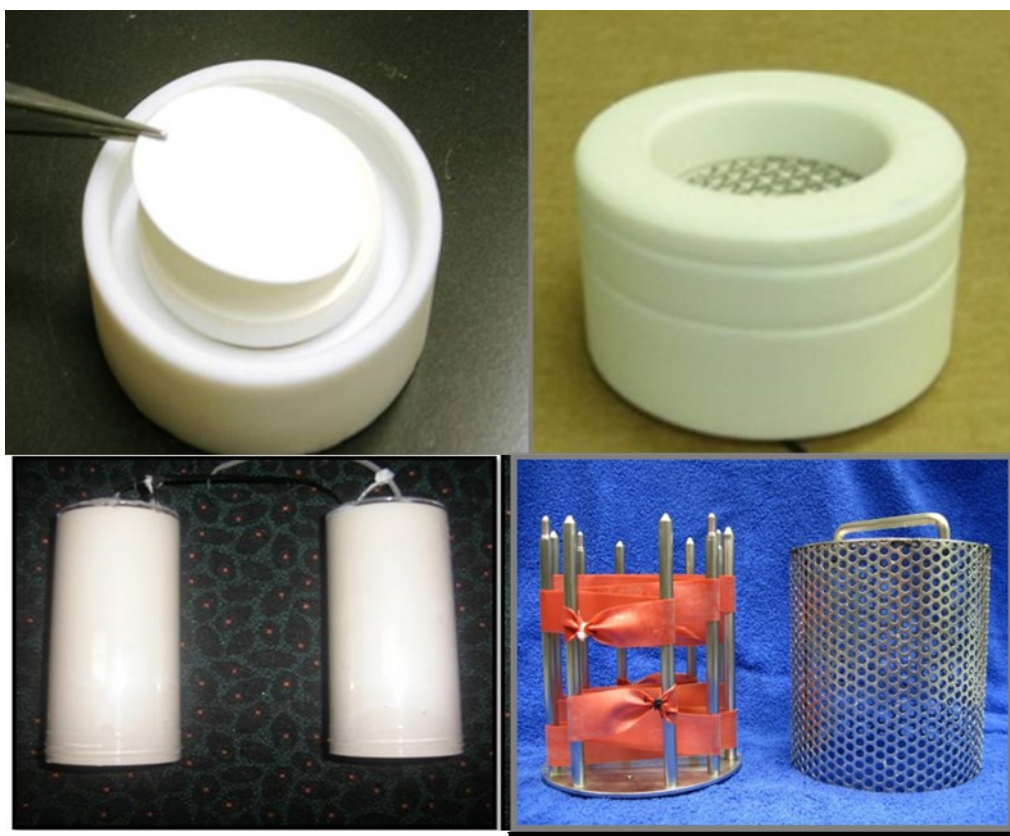
Figure S2 Assembly of Empore Disks (EDs) into Chemcatcher passive sampler housing (top left and right), Passive Flow monitors (PFMs) co-deployed with passive samplers (bottom left) and PDMS passive sampling strips loaded into marine cages (bottom right)
