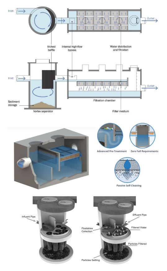
**Figure 6.17 Units based on filtration: Top**: Vortex-separated runoff enters a <u>down-flow cartridge</u> <u>filter system</u>; from above (uppermost) and in profile (below) (Woods Ballard et al. 2015 with courtesy of CIRIA). **Middle**: An <u>up-flow cartridge filter</u> (Courtesy of Bio Clean). **Bottom**: Example of a <u>hollow</u> <u>fibre membrane cartridge filtration system</u> (Courtesy of Contech ES).
