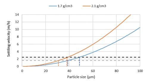
**Figure 6.7** Estimated settling velocities of TWP with density of 1.7 g/cm³ or 2.1 g/cm³ at 10°C in freshwater. The grey and black dashed lines indicate the dimensioning surface load of 1.6 m/h and the maximum dimensioning load of 2.5 m/h, respectively. The calculations for the settling velocities and associated assumptions are described in **Appendix J**.
