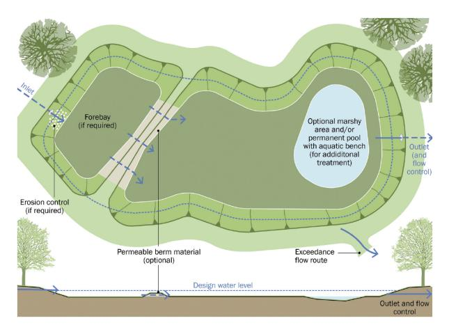
**Figure 5.5** Typical plan view and profile for the design of a dry pond (Woods Ballard et al. 2015 with courtesy of CIRIA).
