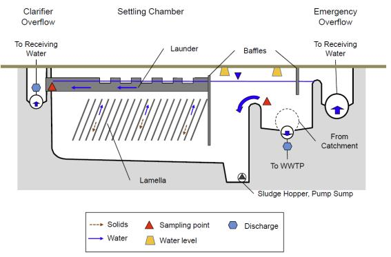
**Figure 6.15.** *Gravitational settling units. Upper:* Schematic of a closed wet basin (translated from Åstebøl (2007). *Middle*: A closed settling tube system (Courtesy of Basal). *Bottom*: Schematic of a lamella settler treating stormwater runoff with discharge of settled sediments to central WWTP and treated water to the aquatic environment (reproduced from Fuchs et al. 2014 with permission from the copyright holders, IWA Publishing).
