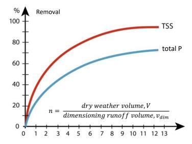
**Figure 5.6** Expected removal of TSS and total phosphorous (total P) as a function of the relationship between the dry weather volume of the permanent pool of a wet sedimentation pond and the dimensioning runoff volume (Statens vegvesen 2014B).
