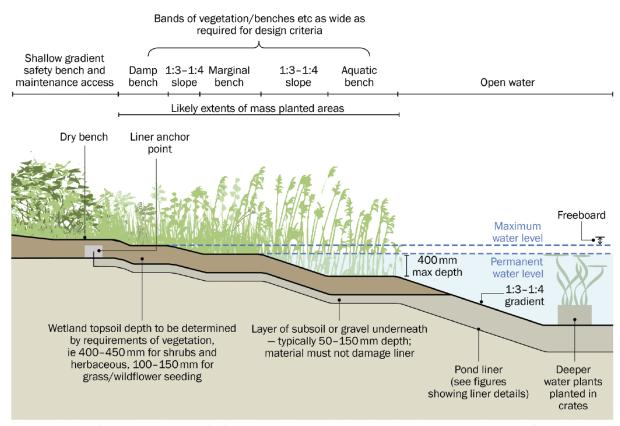
Notes: Width, surfacing and extent etc of safety bench and maintenance access all dependent on site, size of pond, maintenance requirements etc
