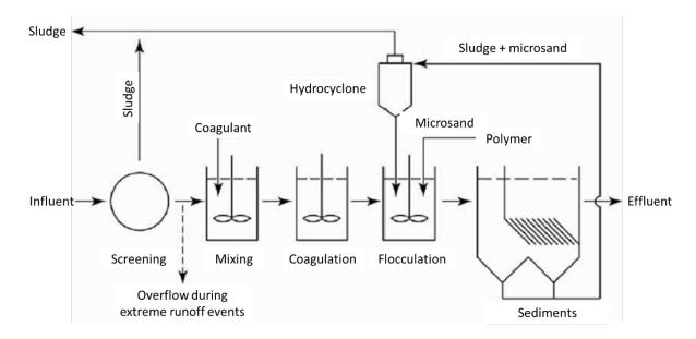
**Figure 6.16 Chemically enhanced settling units**. Schematic drawing of a version of the ballast flocculation process (translated to English from Åstebøl 2007).
