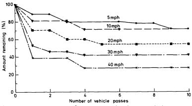
**Figure 12.** Resuspension of 12  $\mu$ m particles due to turbulence generated by a medium size car at various speeds (Nicolson and Branson, 1990)
