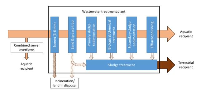
**Figure 6.5** Possible pathways through the sewer system to aquatic and terrestrial environments.
