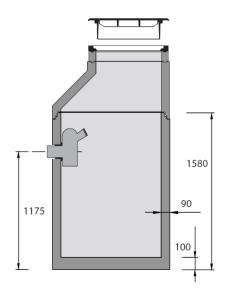
**Figure 6.2** Typical design of a Norwegian roadside gully pot (Courtesy of Basal). The minimum inner diameter is 1000 mm.
