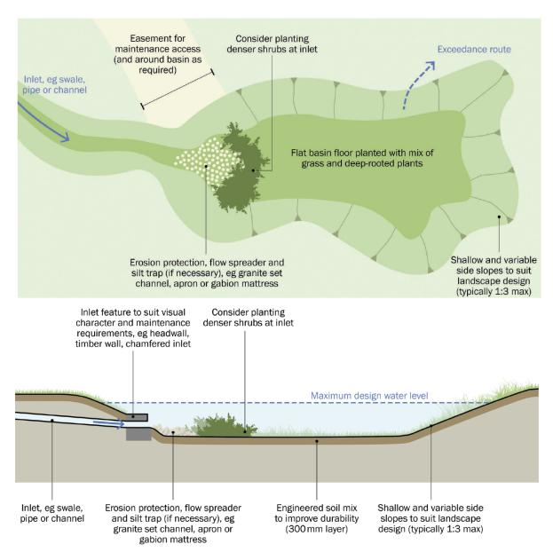
**Figure 5.8** Principle drawing of an infiltration basin from above when it is empty (upper) and in profile when it is filled (below) (Woods Ballard et al. 2015 with courtesy of CIRIA). Note that just a simple forebay is not adequate, according to the revised version of Handbook N200 (Statens vegvesen 2017).
