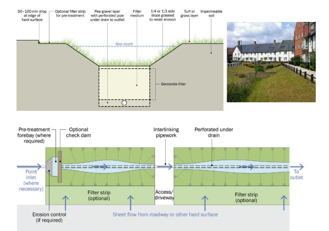
**Figure 6.11** Schematic design of a **dry swale** in profile (upper) and plan view (below) (Woods Ballard et al. 2015 with courtesy of CIRIA; photo: Peterborough City Council).
