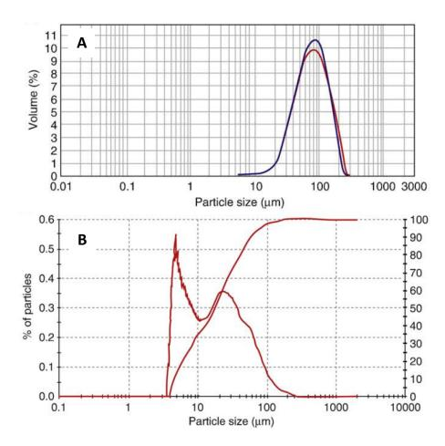
**Figure D1** <u>Volume size distribution</u> (**A**) and <u>number size distribution</u> (**B**) of tread wear particles (TWP) as determined by transmission optical microscopy of samples collected during a run road simulation tests with summer friction tyres on standardized asphalt. Reprinted from Kreider et al. (2010) with permission from Elsevier.
