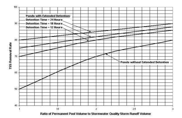
**Figure 5.7** Correlation between expected TSS removal rate (in %) and the ratio between the permanent pool volume and the stormwater runoff volume for wet ponds. The extended detention time curves indicate the available time for additional settling between rainfall events. (NJDEP 2014).
