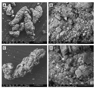
**Figure 2.3** Scanning electron microscope images of RP (A, B) and TWP (C, D). Scales are located below the photos. Mineral incrustations are evident in the photos of greater magnification (B, D). Reprinted from Kreider et al. (2010) with permission from Elsevier.
