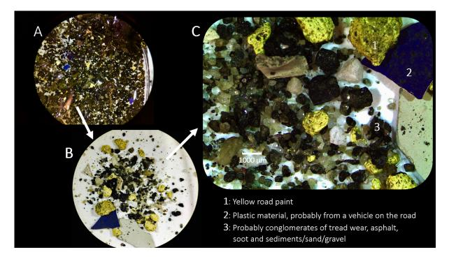
**Figure 2.4** Wear particles of road marking collected from road dust in March 2017 in the Microtyre project. A: The original collected particulates before any separation; B: A collection of micro-, meso-and macro-plastic particles after clean-up; C: Close-up of a section of B). Credit: David Pettersen Eidsvoll, NIVA.
