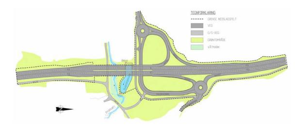
**Figure 2.5** The Skullerud junction and stormwater treatment basins below (a closed sludge basin of  $68 \text{ m}^2$  and an open main basin of  $910 \text{ m}^2$ ) (Åstebøl and Coward 2005).
