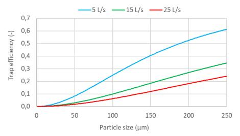
**Figure 6.3** Estimated efficiencies of a gully pot to trap particles with diameters between 1  $\mu$ m and 350  $\mu$ m and a density of 1.7 g/cm<sup>3</sup>when the influent flow velocity to the gully pot is 5-25 L/s. The gully pot has an inner diameter of 1 m.
