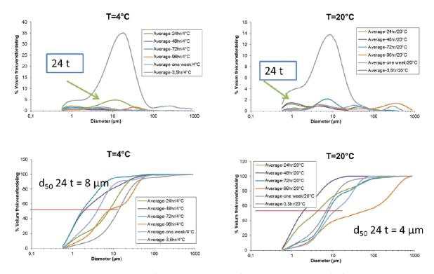
**Figure 7.1** Particle size distribution (as in concentration frequency distribution) after sedimentation at 4 and 20°C (Garshol et al. 2015).
