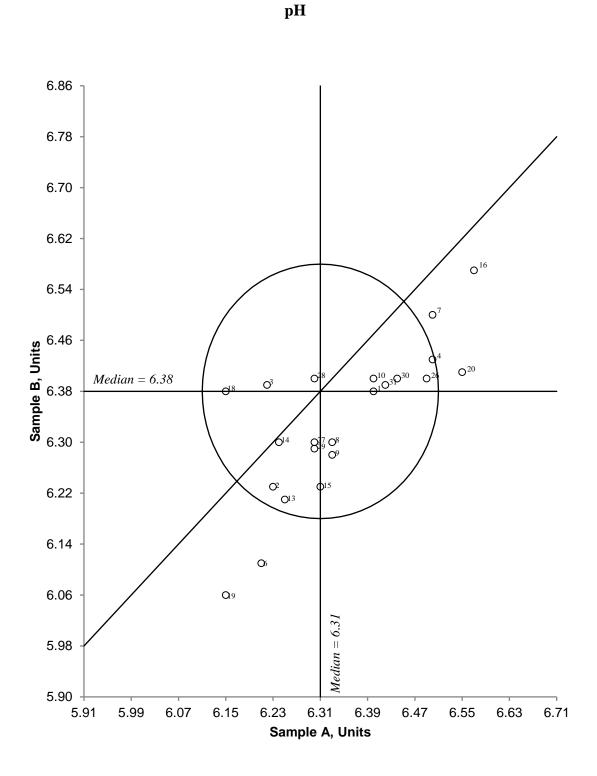
Figure 1. Youden diagram for pH. Sample pair AB. Acceptance limit, given by circle, is 0.2 pH units. (3,15%)
