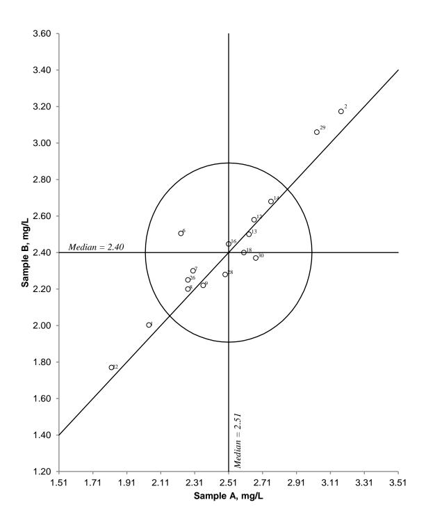
**Figure 11.** Youden diagram for total organic carbon. Sample pair AB. Acceptance limit, given by circle, is 20%.
