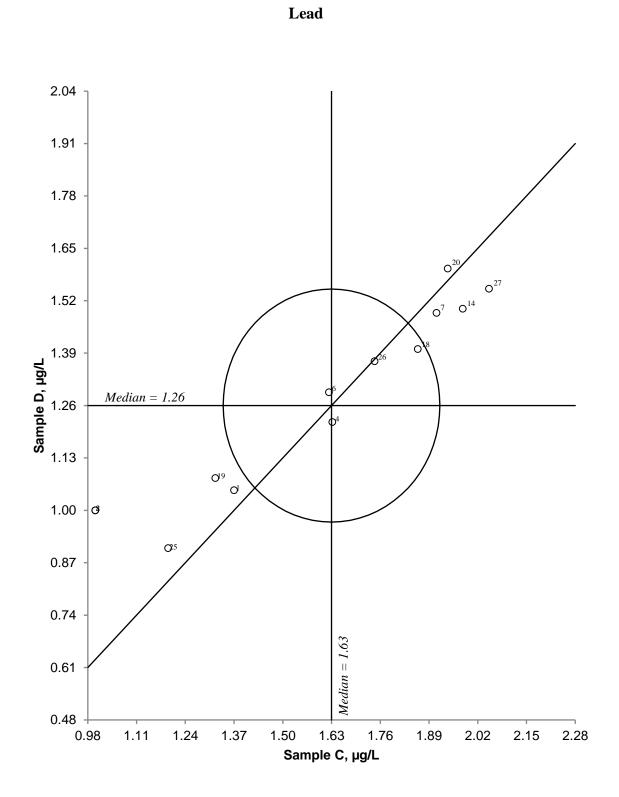
Figure 17. Youden diagram for lead. Sample pair CD. Acceptance limit, given by circle, is 20%.
