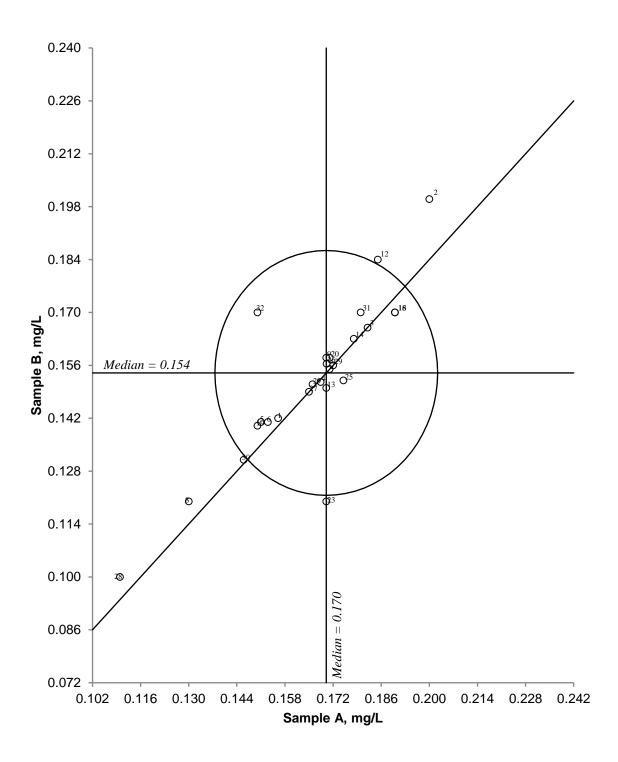
Figure 8. Youden diagram for magnesium. Sample pair AB. Acceptance limit, given by circle, is 20%.
