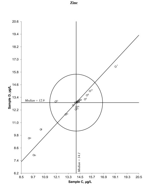
Figure 20. Youden diagram for zinc. Sample pair CD. Acceptance limit, given by circle, is 20%.
