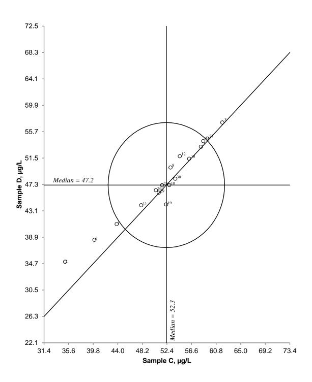
Figure 13. Youden diagram for aluminum. Sample pair CD. Acceptance limit, given by circle, is 20%.
