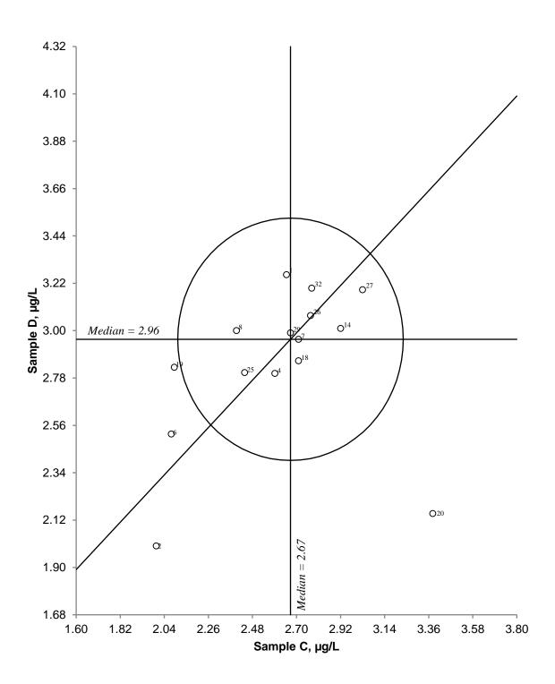
Figure 15. Youden diagram for manganese. Sample pair CD. Acceptance limit, given by circle, is 20%.
