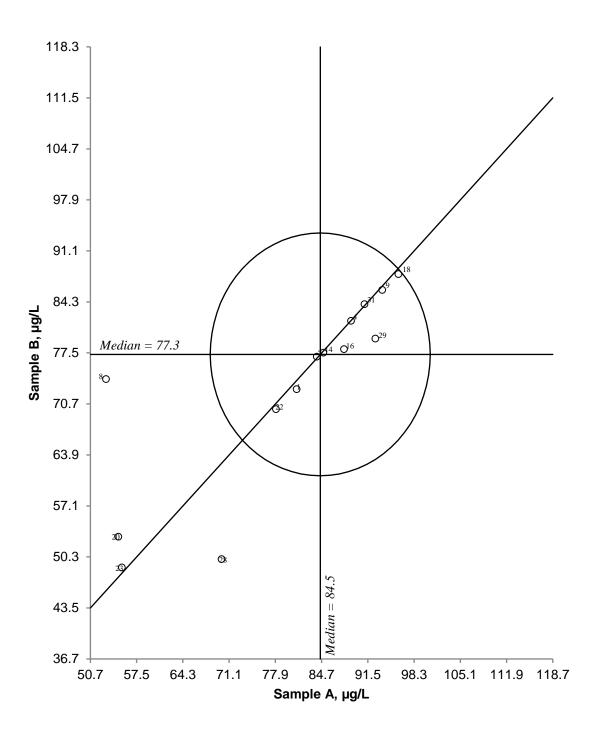
**Figure 4.** Youden diagram for nitrate+nitrite-nitrogen. Sample pair AB. Acceptance limit, given by circle, is 20%.
