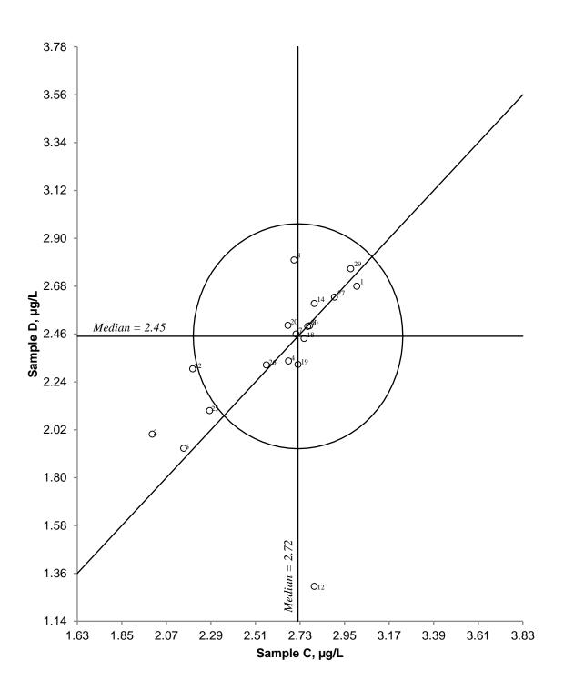
Figure 19. Youden diagram for nickel. Sample pair CD. Acceptance limit, given by circle, is 20%.
