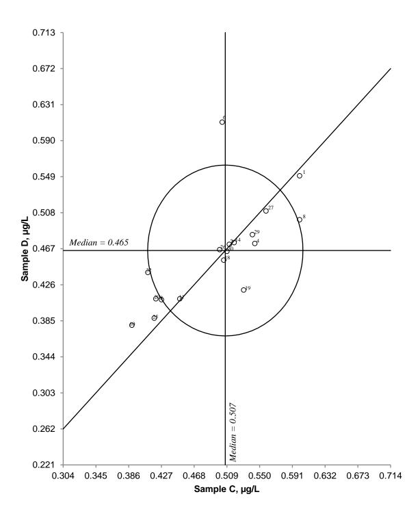
Figure 16. Youden diagram for cadmium. Sample pair CD. Acceptance limit, given by circle, is 20%.
