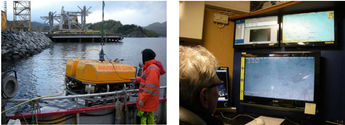
Figure 4: Left: The Argus Mariner ROV from Amundsen Diving which was used during the registrations 26 th -27 th of May 2015. Right: The control room of parent vessel MS Scuba where the ROV pilot sits and where the recordings and records were made.
