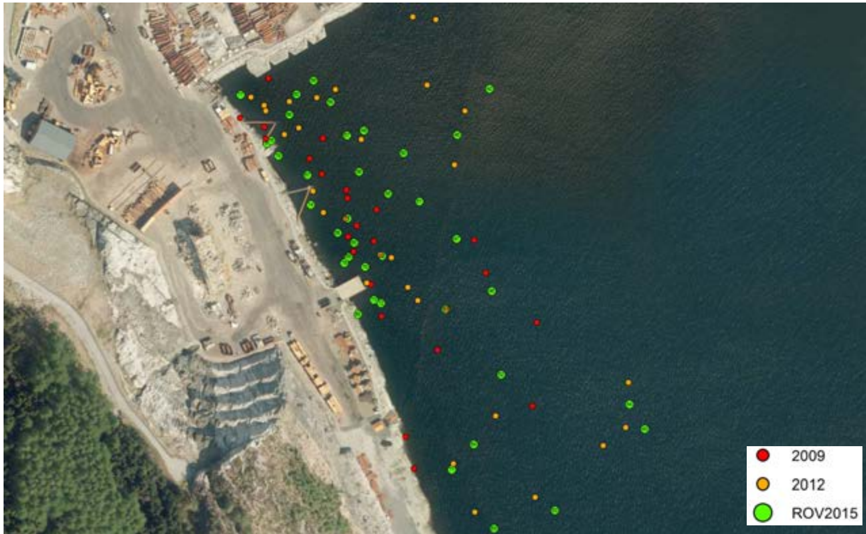
Figure 9: This picture shows the positions of all anthropogenic materials that have been registered and positioned in the area Grønnavika (south of the main quay) during the ROV surveys conducted in 2009, 2012 and 2015. For data registered in 2015, each individual debris object is given an ID number which also is referring to the observations summarised in Table 2.
