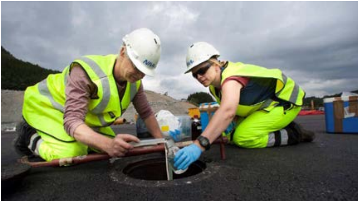
Figure 10: This picture shows how groundwater samples for analysis of contaminant levels were collected from four wells in the quay deck.
