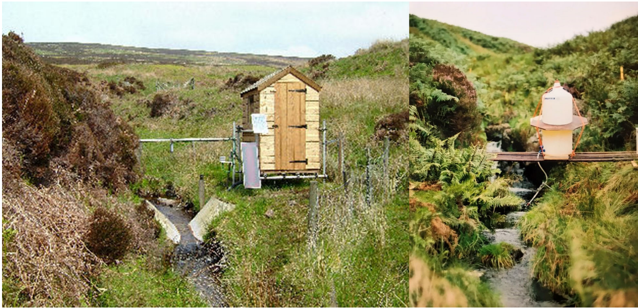
Figure 1. Landscape view of the Birnie Burn (reference stream) and sucrose addition using a 60-L Mariotte bottle in the Cairn burn (treatment stream), Glensaugh research station, north-east Scotland, UK.
