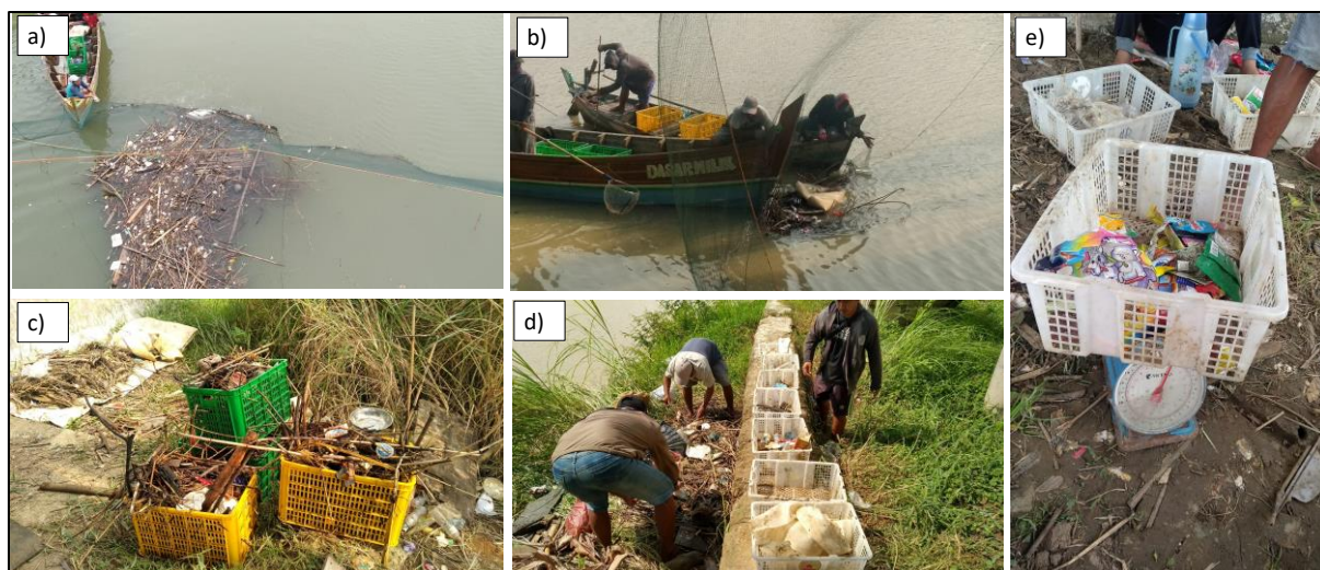
Figure 3. a) the trapping of the debris, b) the manual collection process, c) The collected samples in boxes, d) the sorting process of the samples, e) weighing process of the sorted samples.
