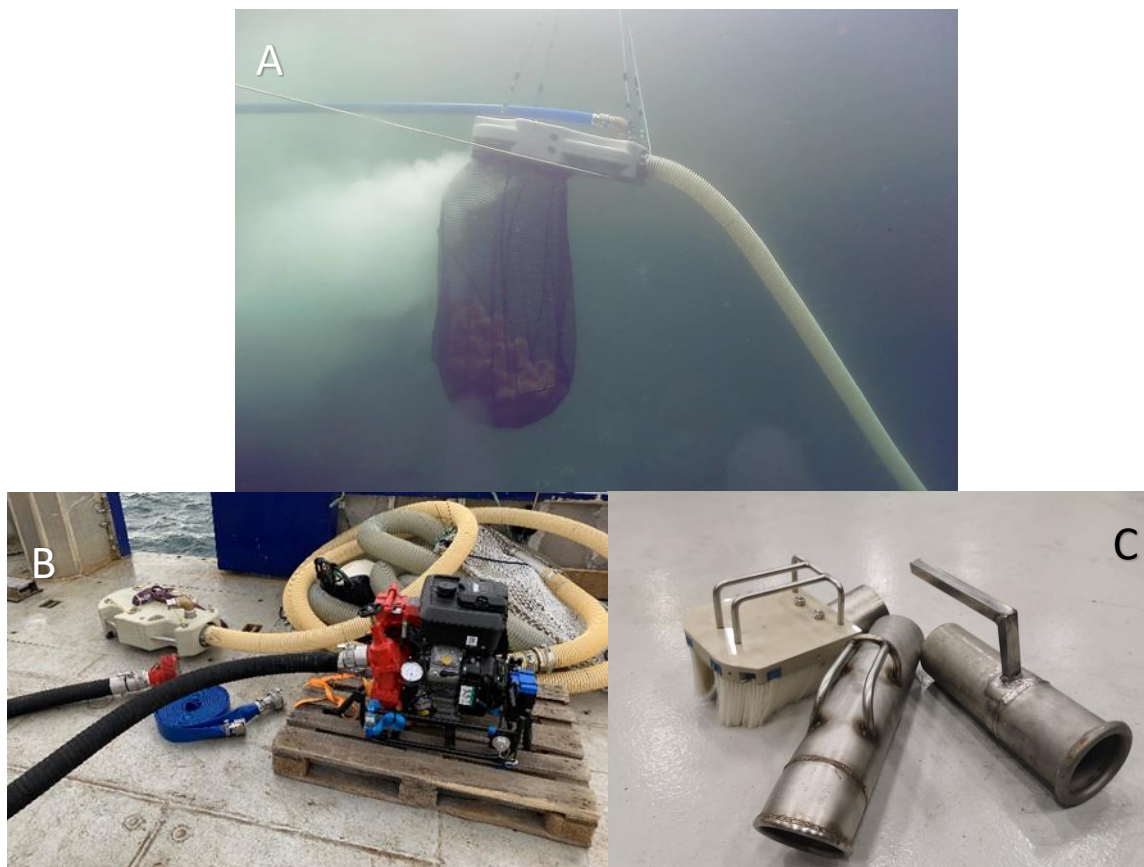
Figure 1. The C disc components with (A) the fire hose, water diverter and the collection bag attached hanging in the water, (B) the water pump that provides the suction and the attached hoses and (C) the nozzles. Photos (A) and (C) by C robotics and photo (B) by NIVA (Helena Michelsen).
