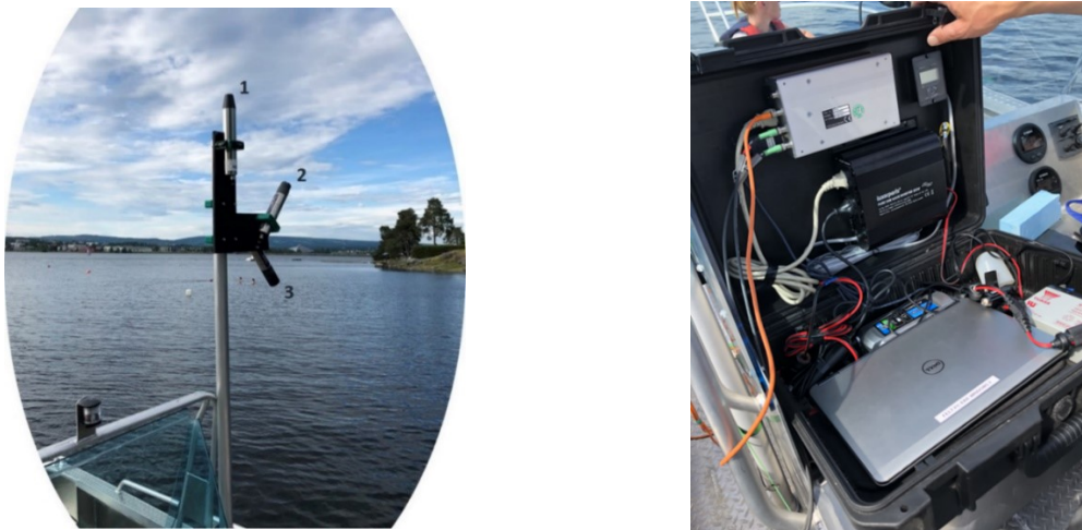
Figure 5. Set up of the rig and computer with TriOS RAMSES light sensors measuring the above reflectance for Mjøsa, 1) Irradiance sensor; incoming light, E_d 2) downwelling, L_d and 3) radiance sensor; upcoming light, L_u . Photo: Sørensen/NIVA.
