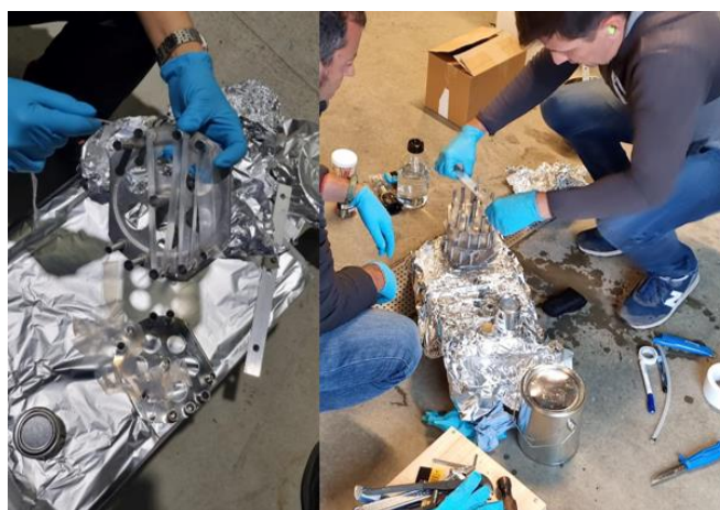
Figure 7 Installation of silicone samplers onto spider holders.
