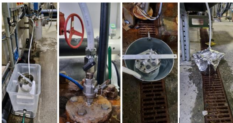
Figure 6 Typical installation of silicone passive samplers mounted on spider holders placed in exposure cells made of a stainless-steel bucket and covered with aluminium.
